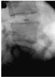
Figure 3. Radiograph with implanted pressure transducer approximately in the center of the L4–L5 nucleus pulposus.
